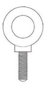
The Tannoy VS10BP loudspeaker can be flown with high quality VEB M10 eyebolts with collar to BS4278:1984. The loudspeaker is equipped with internal steel braces, which also double as the flying points, and accept VEB M10 eyebolts.
