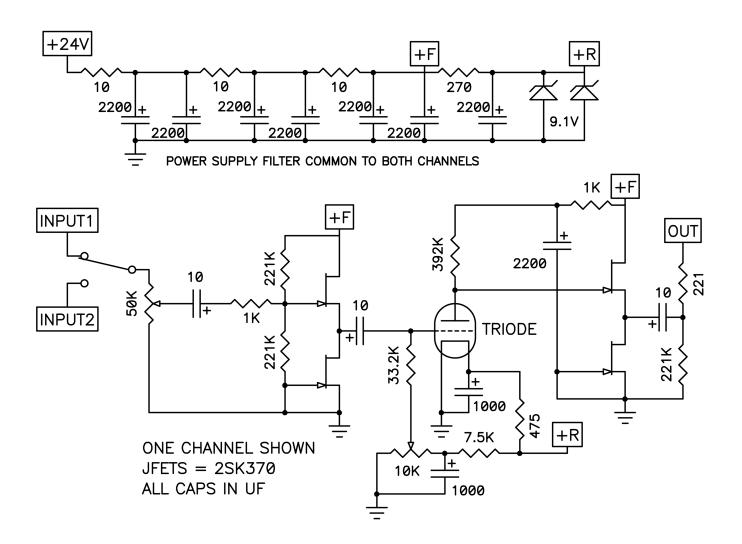
I experimented with numerous values, particularly the plate load resistor, looking for the optimal value for this circuit. I finally used 332 Kohm (please ignore the 392 Kohm on the schematic) which had more gain than the 10 dB I wanted but delivered the harmonic quality I was looking for at the higher output levels.
